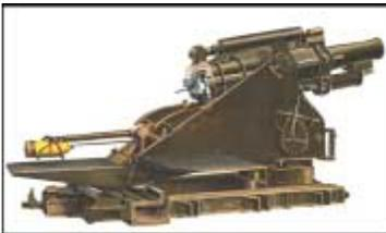
The calibre is the diameter of the barrel. The picture to the left is an example of the heavy artillery that was used in the trenches. The stalemate meant they needed long-range weapons that could deliver devastating blows to the enemy. They needed crews of up to 12 men to work them; the shells weighed up to 900lb –very heavy.
